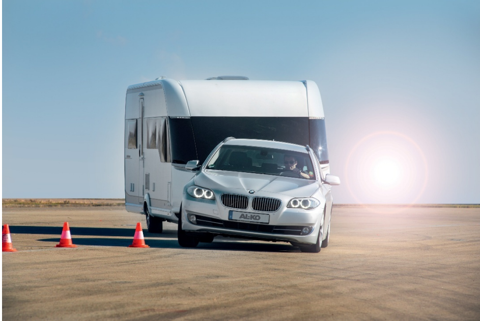
Caption: ATC anti-sway system enhances towing safety © AL-KO VT
