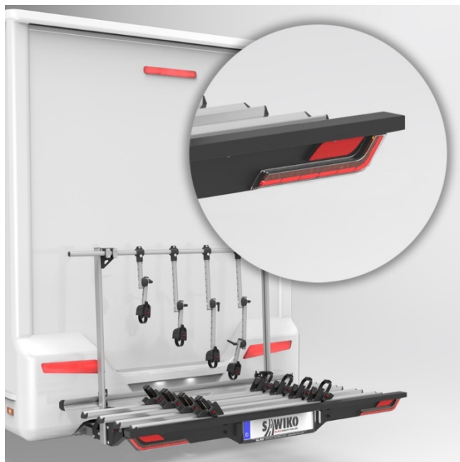
Caption: Integrated LED lighting for VARIO and LIGERO carriers © AL-KO VT
