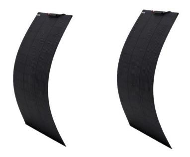
**Caption:** Flexibly capture solar energy: The carrier material and transparent front section of the MFFL150 and the MFFL190 are flexible. Both can adapt to the existing body contours, minimizing the surface area exposed to the buffeting effects of the airstream and both modules of the Flexible Series can be glued on. © AL-KO Vehicle Technology Group
